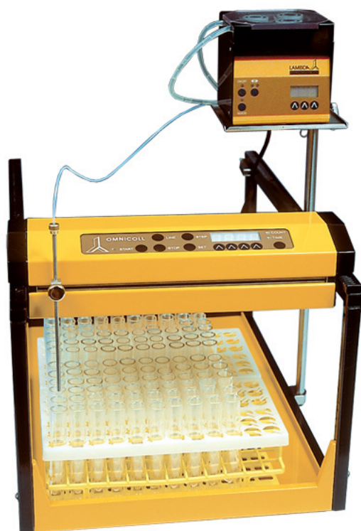
Automated fraction collector and sampler for chromatographic techniques
